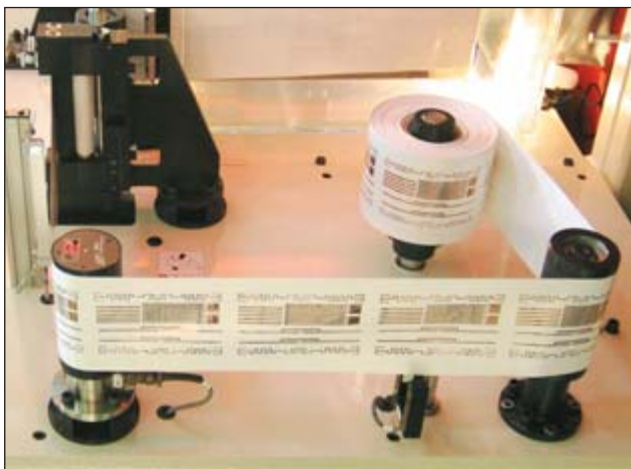
FIGURE 1. Copper circuits on treated PET, created by inkjet.
