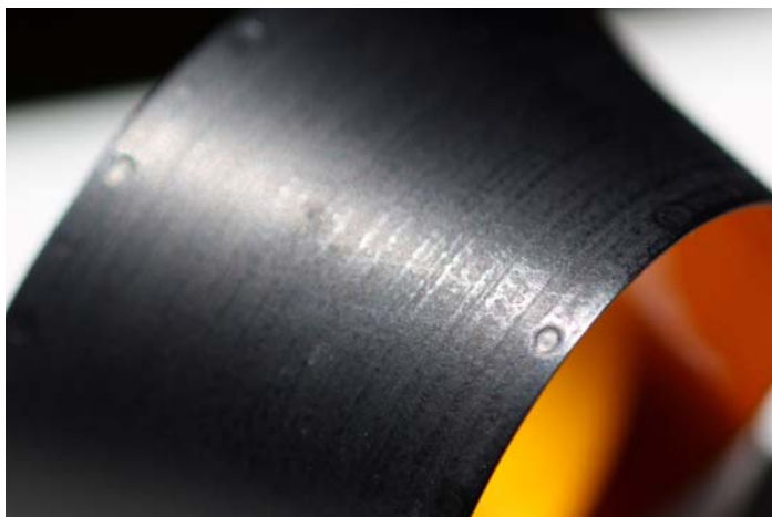
Figure 4- Depressions showing where coverfilm openings allow electrical connection to the shielding film.
