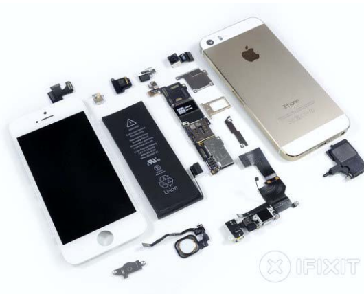
Figure 1 - iPhone 5s teardown by iFixit. Used with permission.
