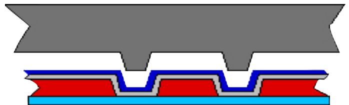
Figure One - Heated roller embosses conductor pattern in base laminate
