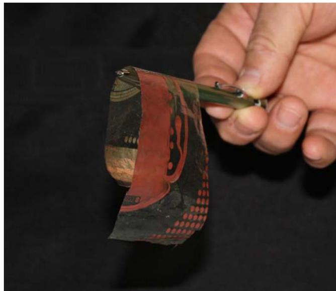
Figure 2 Etched flex draped over a pencil.
